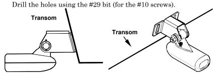
Position transducer mount on transom and mark mounting holes. Side view (left) and shown from above (right).
